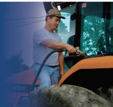
The Ohio Soybean Council and the soybean checkoff are finding new ways to use and improve soybeans. One of those ways being soy biodiesel, a clean-burning, renewable fuel made from soybeans. Most commonly blended with petroleum diesel, soy biodiesel can be used in any diesel engine with no modifications to the engine. Most common blends are B2, B10 and B20 (20-percent biodiesel and 80-percent petroleum diesel).
