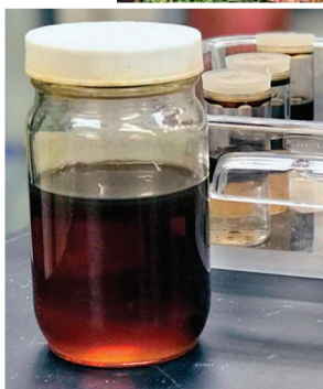
Soy-based cationic surfactant being tested for improved oil recovery applications for existing oil and gas wells.
